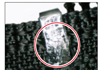
Coil zipper (P-TOP) damage example
