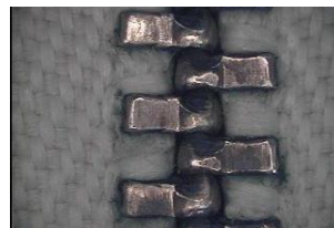
Blackish stain can be observed on the garment fabrics at where the zipper chain was probably attached or pressed on. The stain migration is particularly obvious on the light color.
