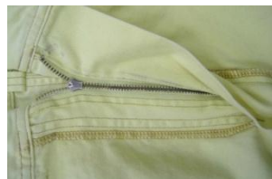
Blackish stain can be observed on the garment fabrics at where the zipper chain was probably attached or pressed on. The stain migration is particularly obvious on the light color.
