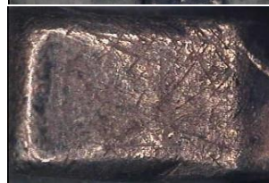
The surface of the metal component e.g. elements are scratched or scraped. The scraped off metal dust may be mixed with the dirt washed off from the garment and cause the staining problem.
