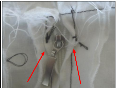
The garment fabric is sewn down to keep away from contact with the slider.
